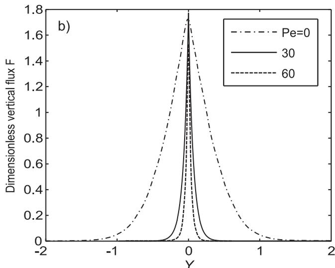
Fig. 3. Vertical heat fluxes along  $X$  (a) and  $Y$  (b) direction at the plane  $Z = 0$  (Fig. 1).  $Pe$  numbers are tuned by changing the Darcy flux, other parameters are fixed. The BHE is located at  $(0,0)$ . GWF: groundwater flow.
