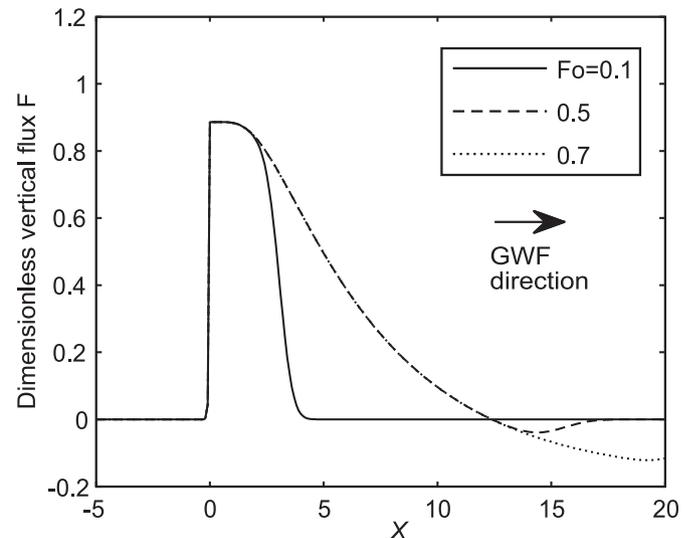
Fig. 7. Vertical heat fluxes along  $X$  direction at the plane  $Z = H$  (see Fig. 1) and  $Pe = 30$ .  $Fo$  numbers are tuned by changing the time, other parameters are fixed. The BHE is located at the origin  $(0,0)$ . GWF: groundwater flow.
