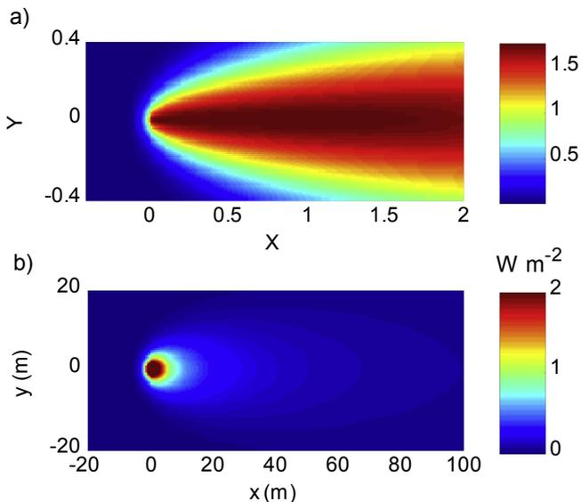
Fig. 2. Vertical heat fluxes at the top boundary at:  $t = 10$  years ( $Fo = 0.1$ ),  $q_d = 9.4 \text{ m y}^{-1}$  ( $Pe = 30$ ); (a) dimensionless magnitudes according to Eq. (9), and (b) absolute values ( $\text{W m}^{-2}$ ) according to Eq. (7). Groundwater flows along the  $x$  direction, borehole length  $H = 50 \text{ m}$ ,  $q = 40 \text{ W m}^{-1}$ . BHE is located at  $(0,0)$ .
