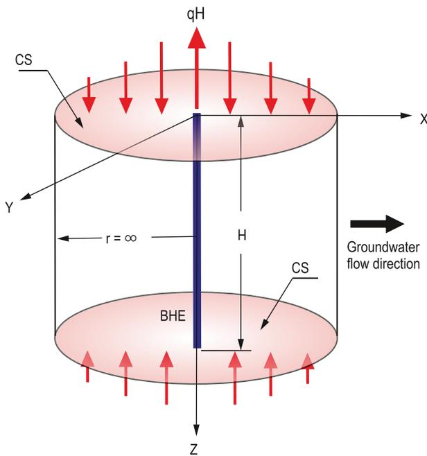
**Fig. 1.** Cylindrical control volume (CV) for heat balance calculation. Red arrows indicate heat fluxes, and  $qH$  is the total power extracted by the BHE. CS denotes the control surface of the CV. (For interpretation of the references to colour in this figure legend, the reader is referred to the web version of this article.)
