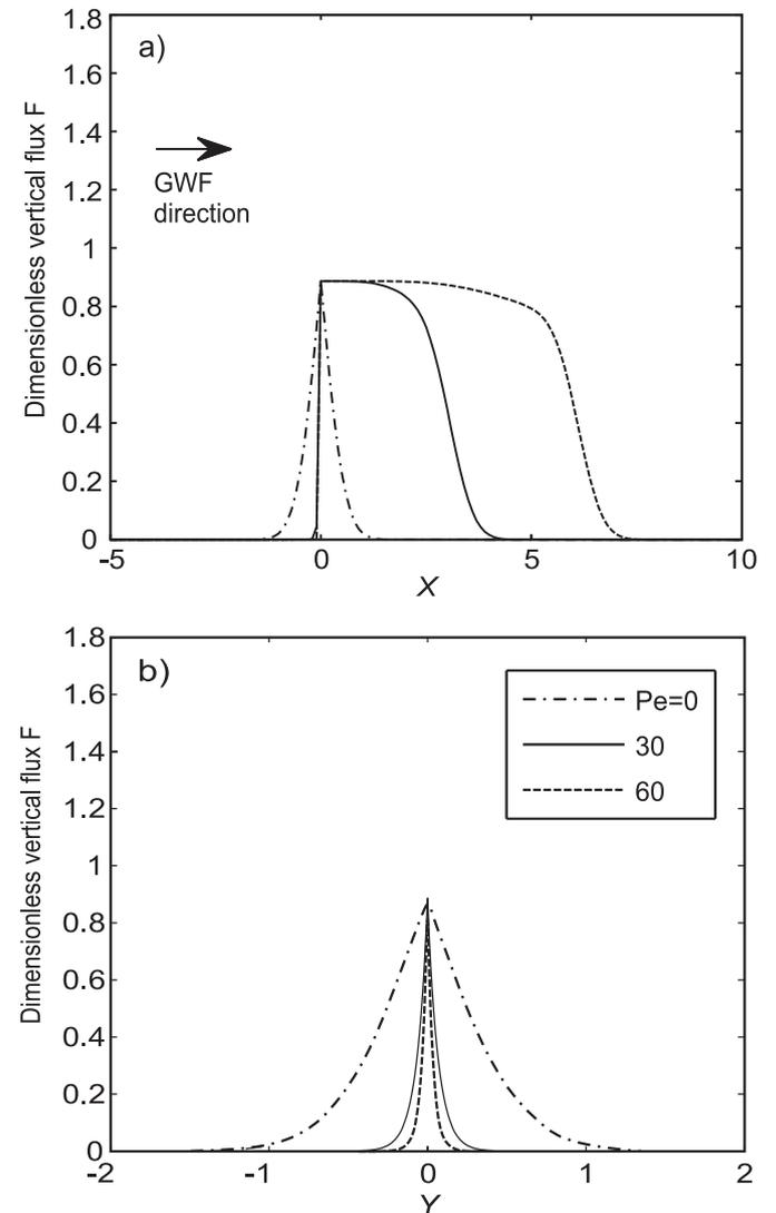
Fig. 5. Vertical heat fluxes along  $X$  (a) and  $Y$  (b) direction at the plane  $Z = H$  (see Fig. 1).  $Pe$  numbers are tuned by changing the Darcy flux, other parameters are fixed. The BHE is located at  $(0,0)$ . GWF: groundwater flow.
