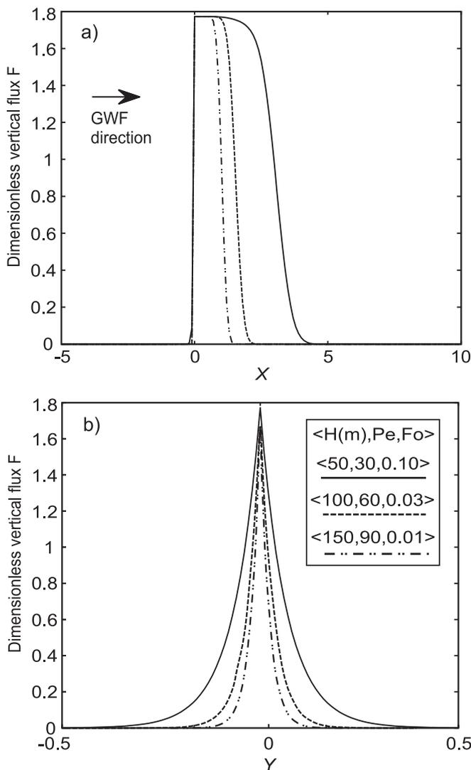
Fig. 4. Vertical heat fluxes along  $X$  (a) and  $Y$  (b) direction at the plane  $Z = 0$  (see Fig. 1).  $Pe$  and  $Fo$  are tuned by changing  $H$ , other parameters are fixed. The BHE is located at the origin  $(0,0)$ . GWF: groundwater flow.
