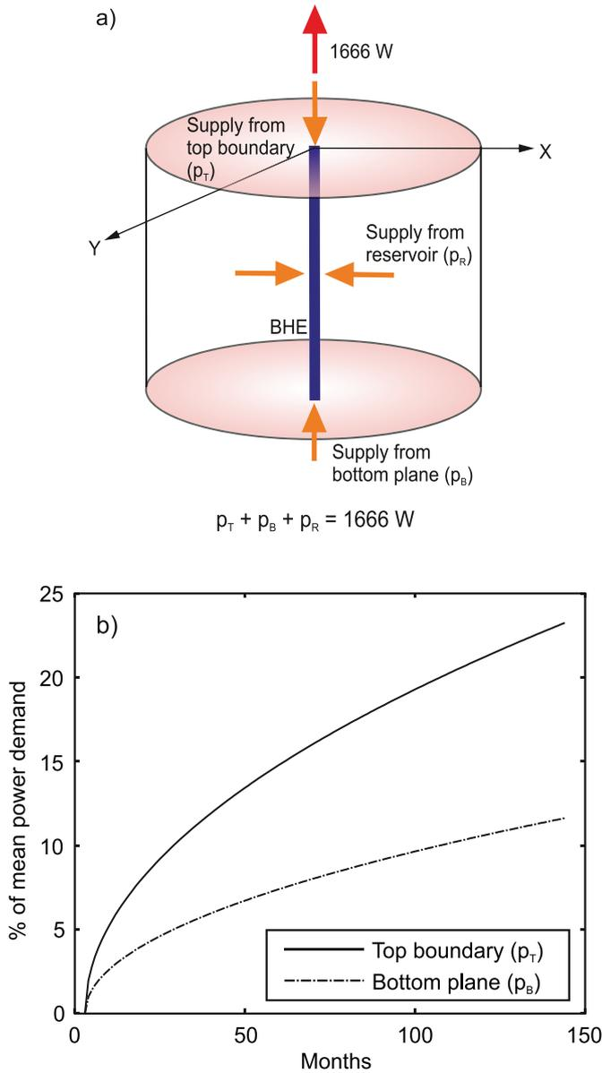
**Fig. 10.** Power balance for the BHE installed at the Elgg site; (a) scheme identifying the heat sources and (b) fractions of the total power demand (%) supplied by the top ( $p_T$ ) and bottom planes ( $p_B$ ).  $p_R$  is the power contribution from the reservoir. The annual mean power demand is 1666 W.
