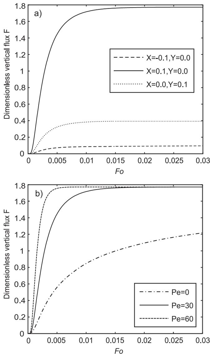
Fig. 6. Vertical heat fluxes in time at  $Z = 0$  for (a) different  $X$  and  $Y$  locations and fixed  $Pe = 30$ . (b) different  $Pe$  (here changing the Darcy flux) and fixed position  $X = 0.1, Y = 0$ .
